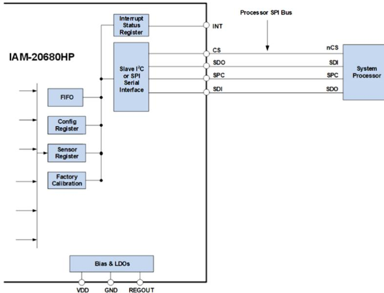
**Figure 7. IAM-20680HP Solution Using SPI Interface**
