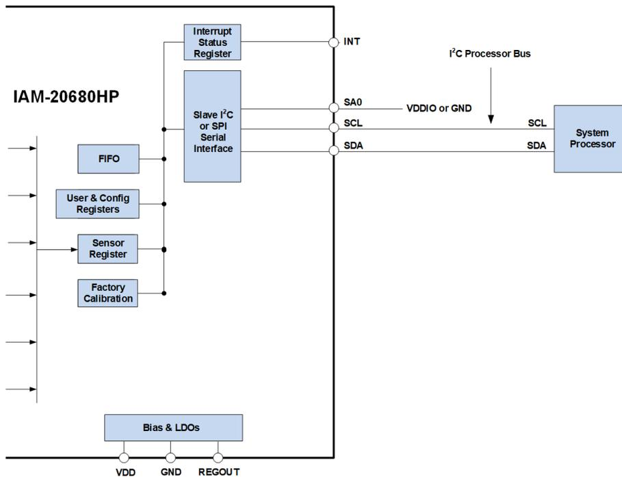
Figure 6. IAM-20680HP Solution Using I<sup>2</sup>C Interface
