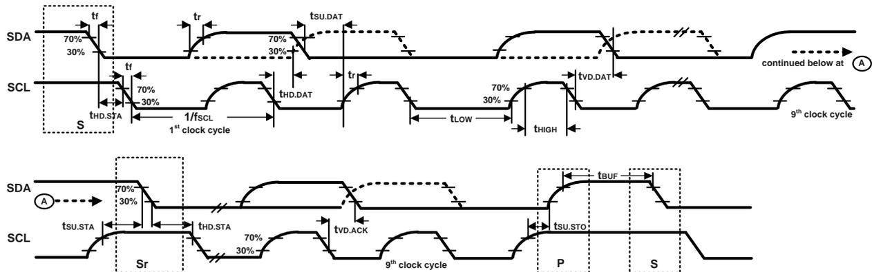
Figure 1. I<sup>2</sup>C Bus Timing Diagram
