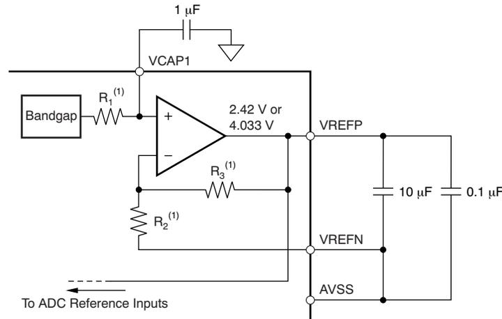
(1) For  $V_{REF} = 2.42\text{ V}$ :  $R_1 = 100\text{ k}\Omega$ ,  $R_2 = 200\text{ k}\Omega$ , and  $R_3 = 200\text{ k}\Omega$ . For  $V_{REF} = 4.033\text{ V}$ :  $R_1 = 84\text{ k}\Omega$ ,  $R_2 = 120\text{ k}\Omega$ , and  $R_3 = 280\text{ k}\Omega$ .
