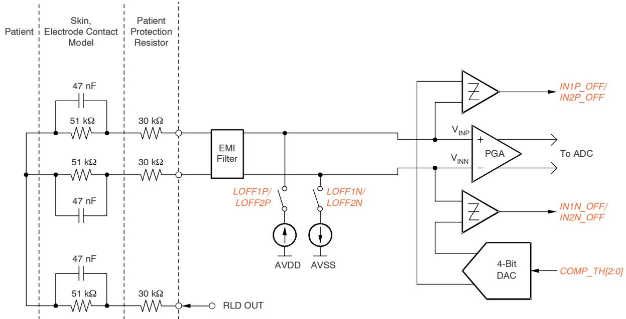
NOTE: The  $R_P$  value must be selected in order to be below the maximum allowable current flow into a patient (in accordance with the relevant specification the latest revision of IEC 60601).
