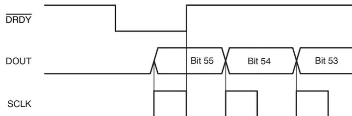
Figure 30.  $\overline{\text{DRDY}}$  with Data Retrieval ( $\overline{\text{CS}} = 0$ )
