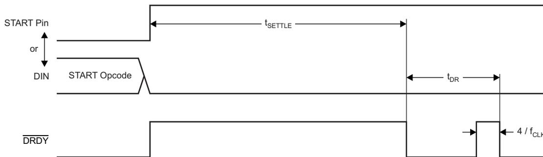
(1) Settling time uncertainty is one  $t_{MOD}$  cycle.
