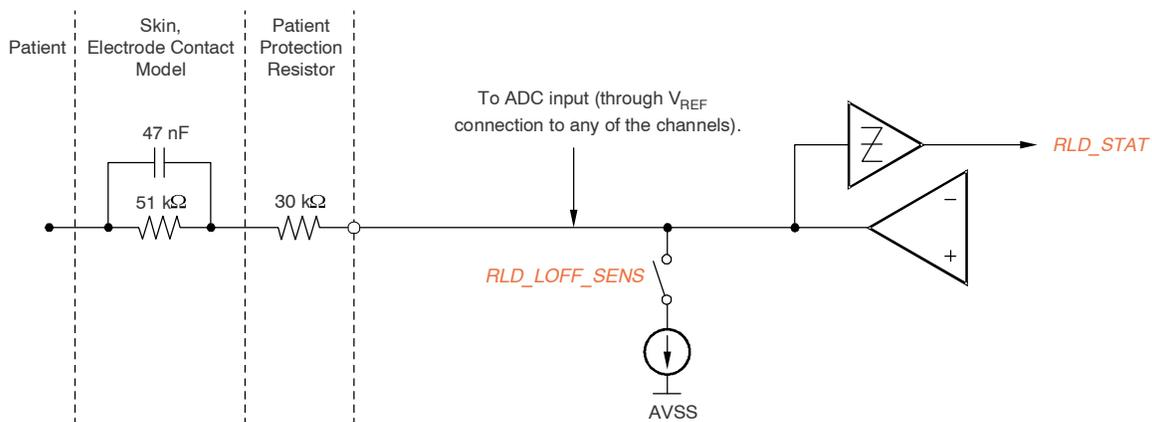
NOTE: The  $R_P$  value must be selected in order to be below the maximum allowable current flow into a patient (in accordance with the relevant specification the latest revision of IEC 60601).
