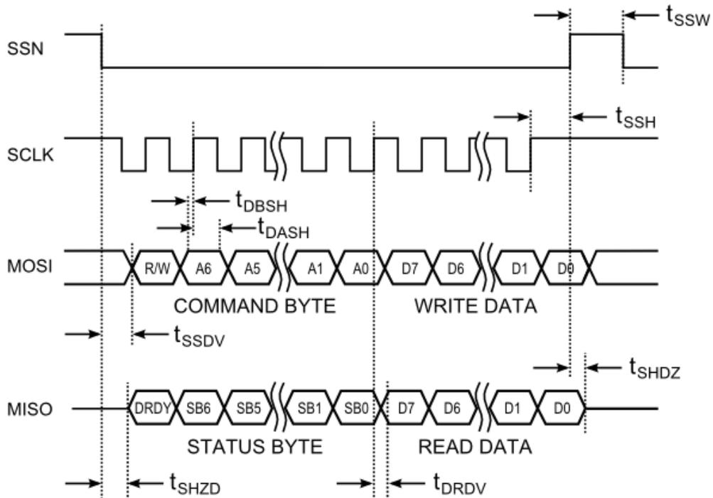
Figure 4-6: SPI Timing Diagram,  $CPOL = CPHA = 1$
