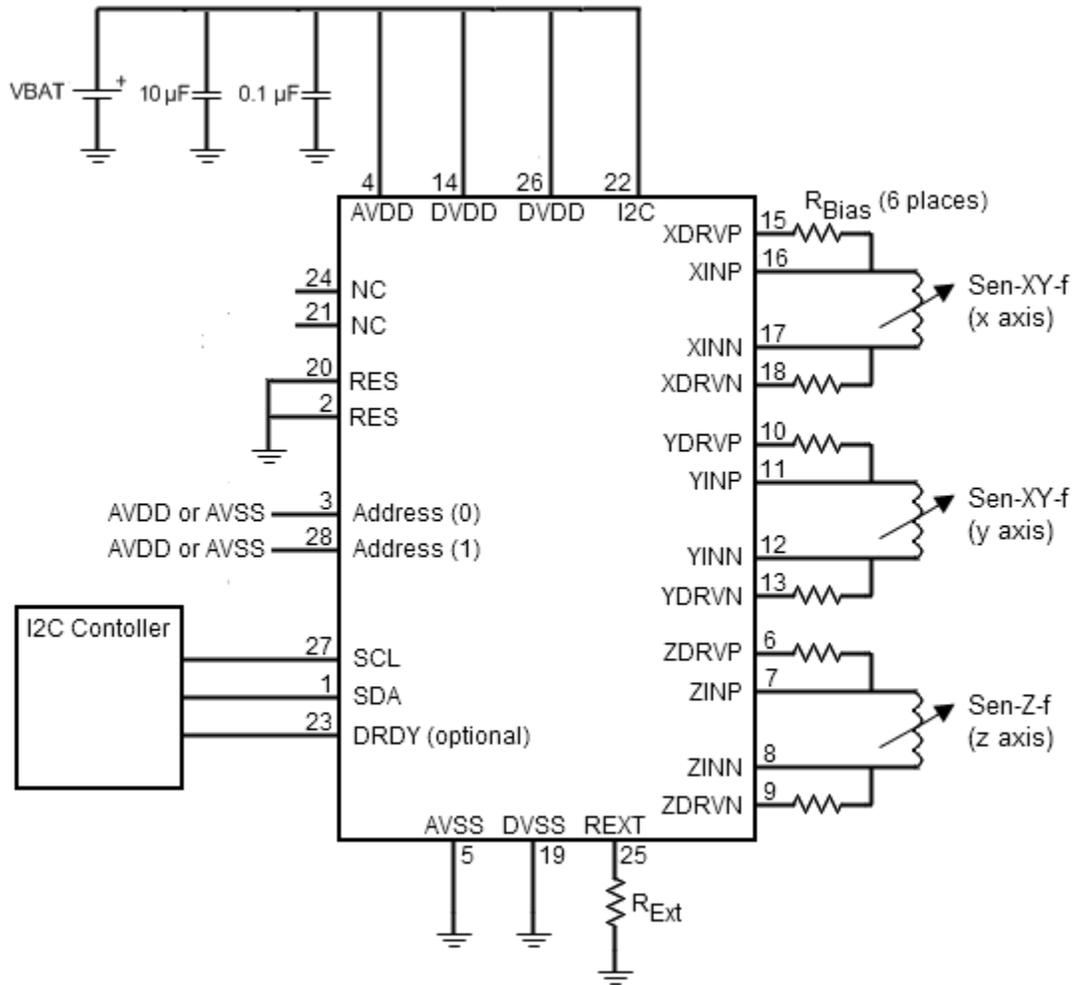
Figure 4-2: RM3100 reference schematic – I<sup>2</sup>C Configuration
