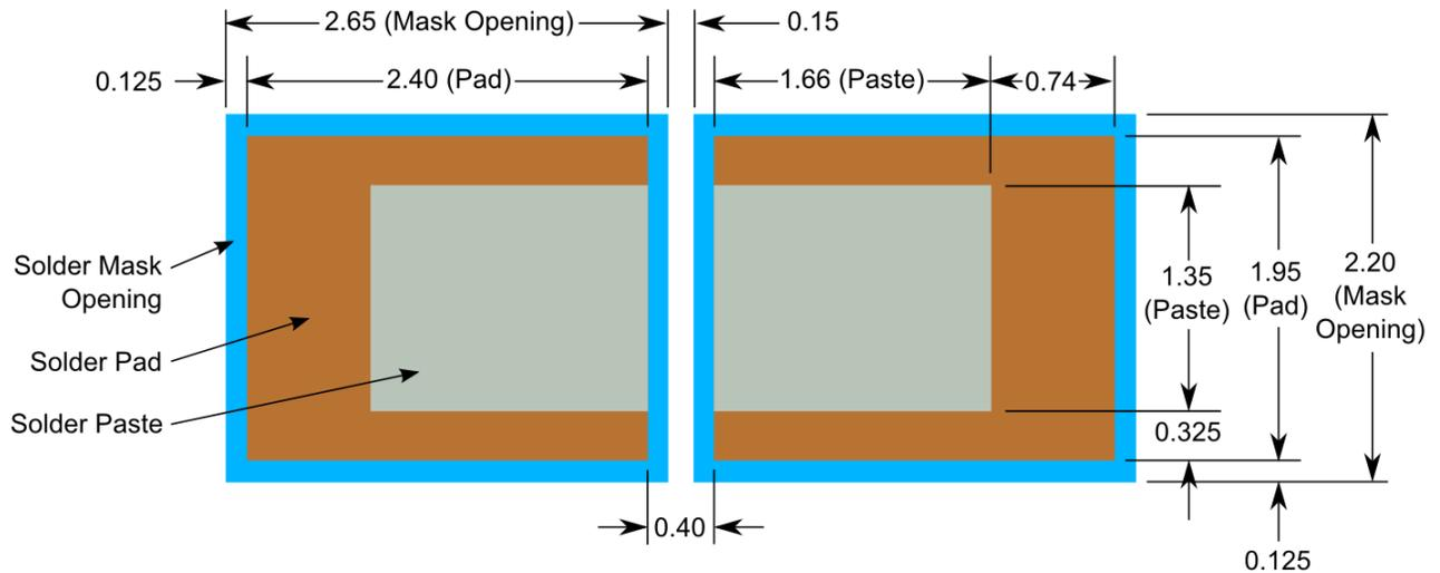
**Note:** PNI recommends a 5 mil stencil. The solder paste area is much smaller than the pad to reduce sensor tilt and misalignment. The above layout allows for rework: for minimal footprint, contact PNI.
