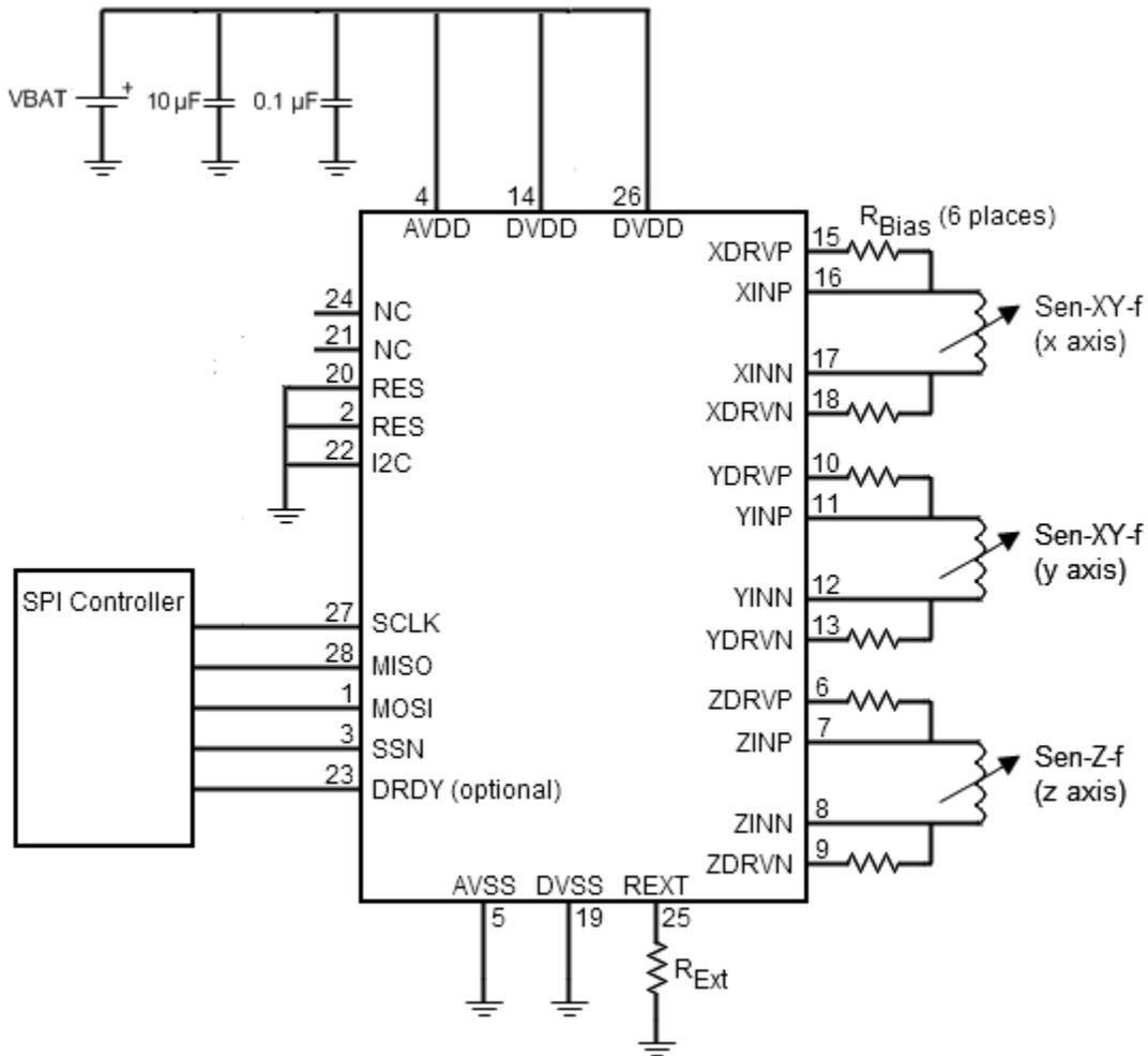
Figure 4-1: RM3100 reference schematic – SPI Configuration
