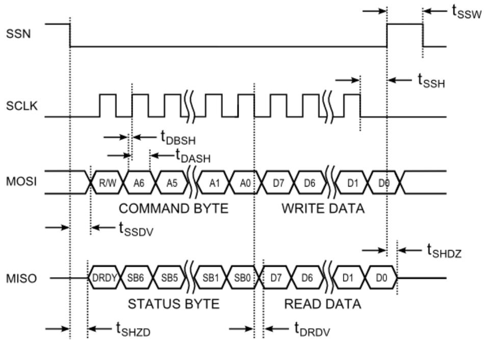
Figure 4-5: SPI Timing Diagram,  $CPOL = CPHA = 0$
