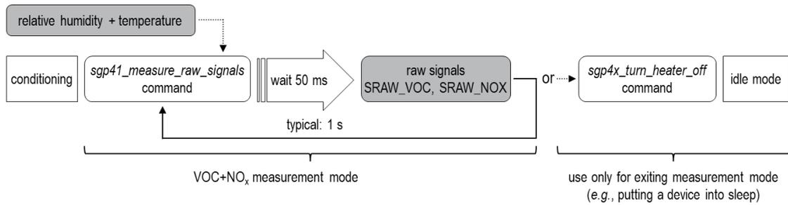
**Figure 9** Process flow for performing a raw signal measurement with the SGP41. For enabling on-chip humidity compensation, current relative humidity and temperature values have to be supplied as part of the measurement command.
