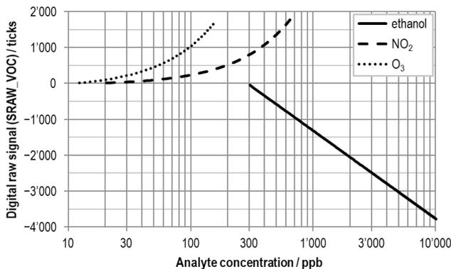
**Figure 2** Typical sensor response by the VOC signal to ethanol, NO<sub>2</sub>, and O<sub>3</sub> normalized to 500 ppb of H<sub>2</sub> + 500 ppb of ethanol. Data were recorded at 25 °C and 50 % RH and a power supply of VDD of 3.3 V.
