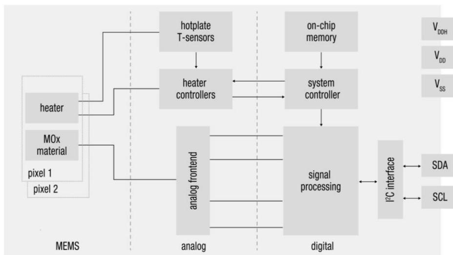
**Figure 1** Functional block diagram of the SGP41.
