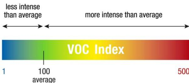
**Figure 11** Explanation of the VOC Index scale.
