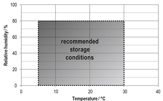
**Figure 5** Recommended relative humidity and temperature for storing the SGP41.
