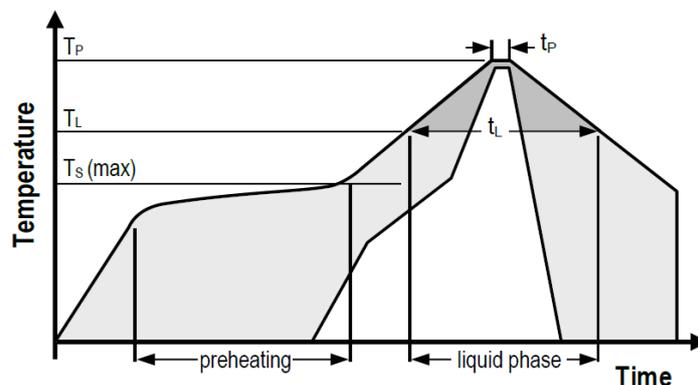
**Figure 19** Soldering profile according to JEDEC standard. Recommended conditions are  $T_P = 245\text{ }^\circ\text{C}$  and  $t_p \leq 30\text{ s}$  for Pb-free assembly,  $T_L < 220\text{ }^\circ\text{C}$  and  $t_L < 150\text{ s}$ . Ramp-up rate  $<3\text{ }^\circ\text{C s}^{-1}$  and ramp-down rate  $<4\text{ }^\circ\text{C s}^{-1}$ .
