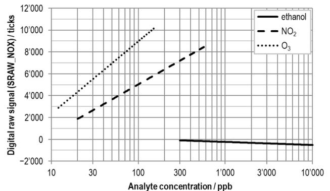
**Figure 3** Typical sensor response by the NO<sub>x</sub> signal to ethanol, NO<sub>2</sub>, and O<sub>3</sub> normalized to 500 ppb of H<sub>2</sub> + 500 ppb of ethanol. Data were recorded at 25 °C and 50 % RH and a power supply of VDD of 3.3 V.
