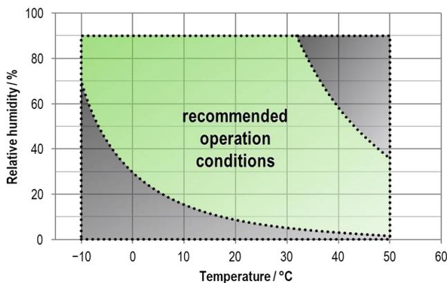
**Figure 4** Recommended relative humidity and temperature for operating the SGP41. Green area marks conditions for which humidity compensation has been optimized. Additionally, gray areas mark operating conditions without using the humidity compensation feature.
