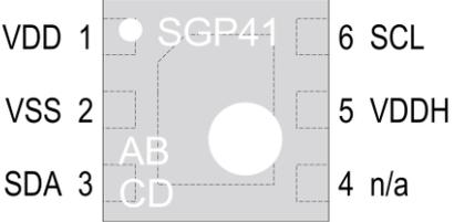
**Table 6** Pin assignment (transparent top view). Dashed lines are only visible from the bottom.
